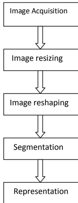
Figure 2.1: Block diagram of Otsu method
