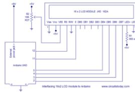
Figure 2.4: Interfacing LCD with Arduino microcontroller
