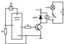
Figure 5.10: Interfacing Relay module with Arduino
