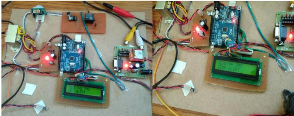
**Fig 6.2: LCD showing “Sending SMS Cry Alert” Fig 6.3: LCD showing “Sending SMS TEMP Alert”**
