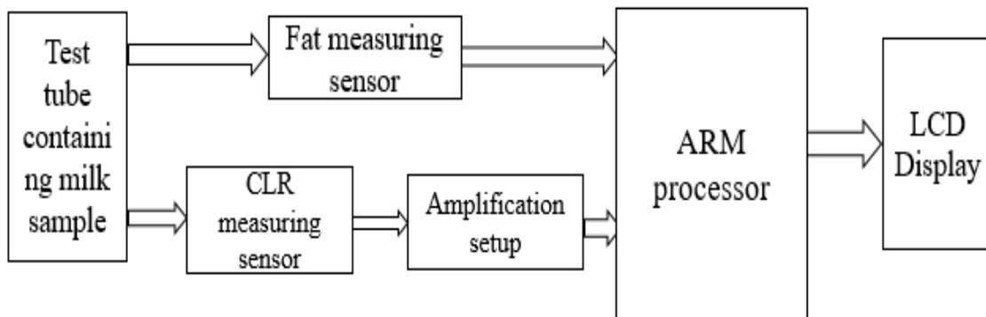
**Figure 2.1: Block Diagram of Advanced Lactotester**
