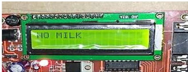
**Figure 3.2: No Milk sample detected**
