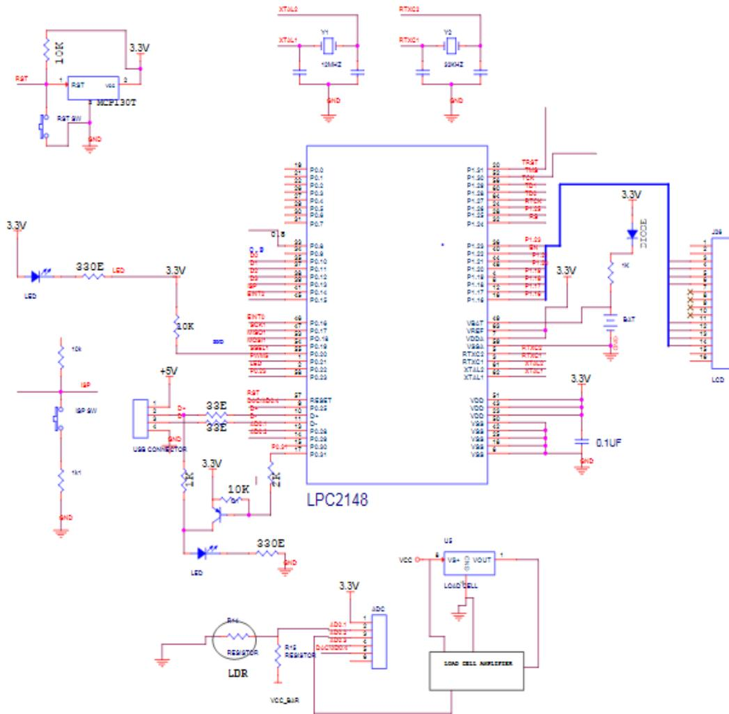
**Fig 2.2. Schematic Diagram for Advanced Lactotester**
