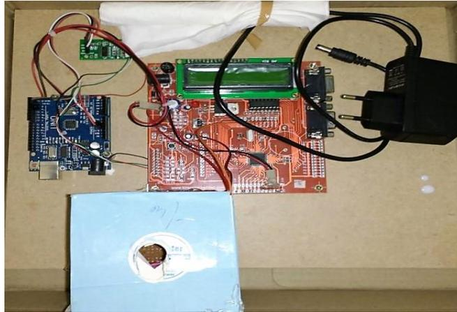
**Figure 3.1: Project Test Setup of Advanced Lactotester**
