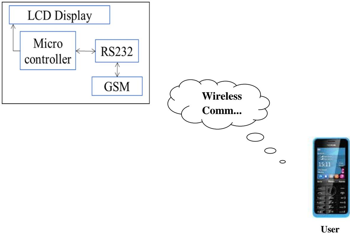
Fig 2: Block Diagram of Bus-Station module
