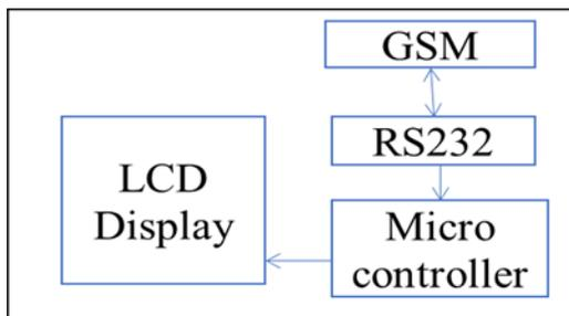
Figure 6: Block Diagram of Bus-Stop Module
