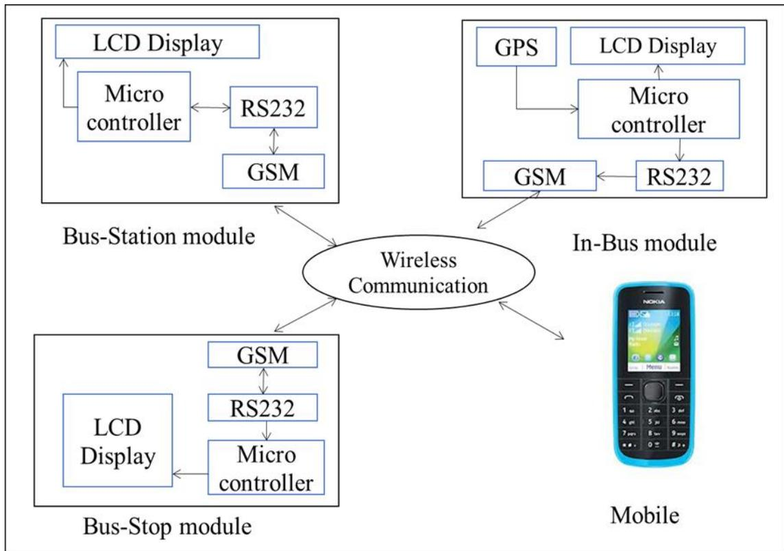
Fig 1: Block Diagram of a GSM-GPS Based Automatic Vehicle Locating System for Bus Transit
