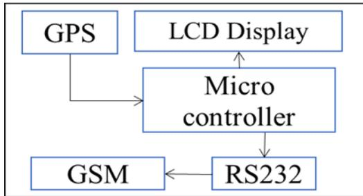
Figure 4: Block Diagram of In-Bus Module
