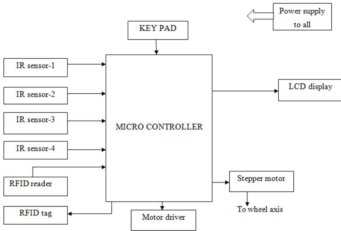
**Figure 1:** Block Diagram of Rotary Automated Car Parking System
