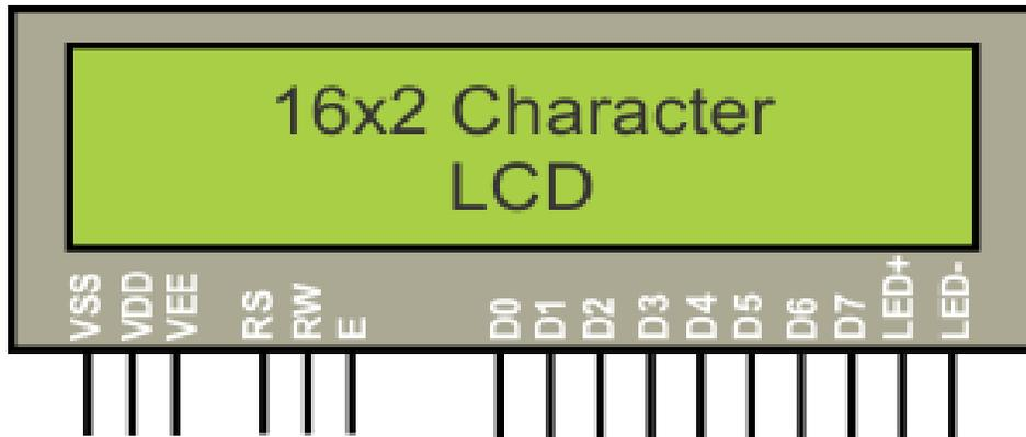
**Figure: Pin Diagram of LCD**
