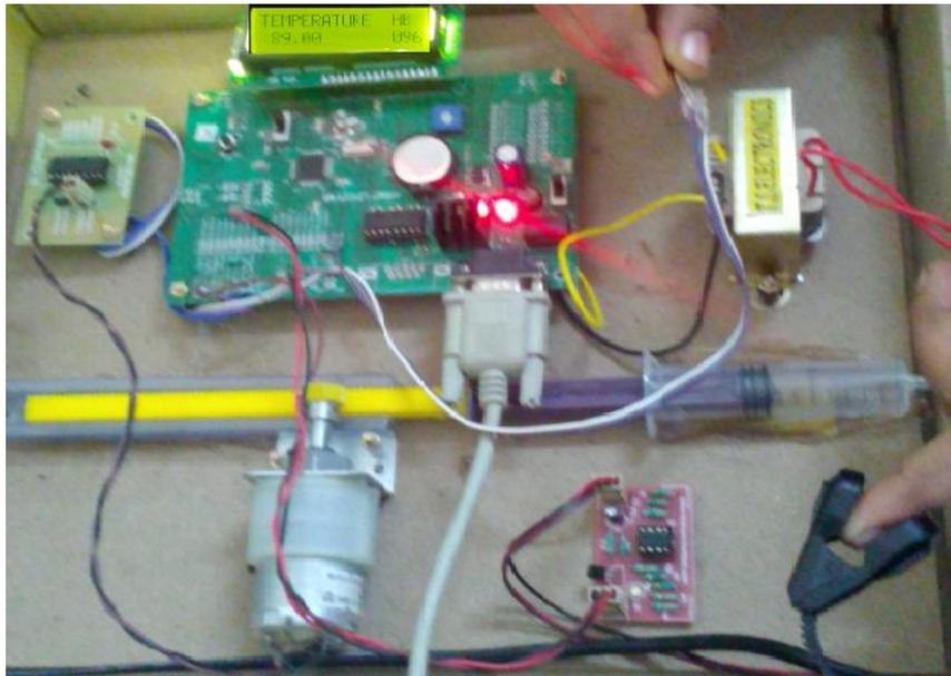
**Figure 5.4:**Physical View of Automatic Anaesthesia Injector using Arm Controller
