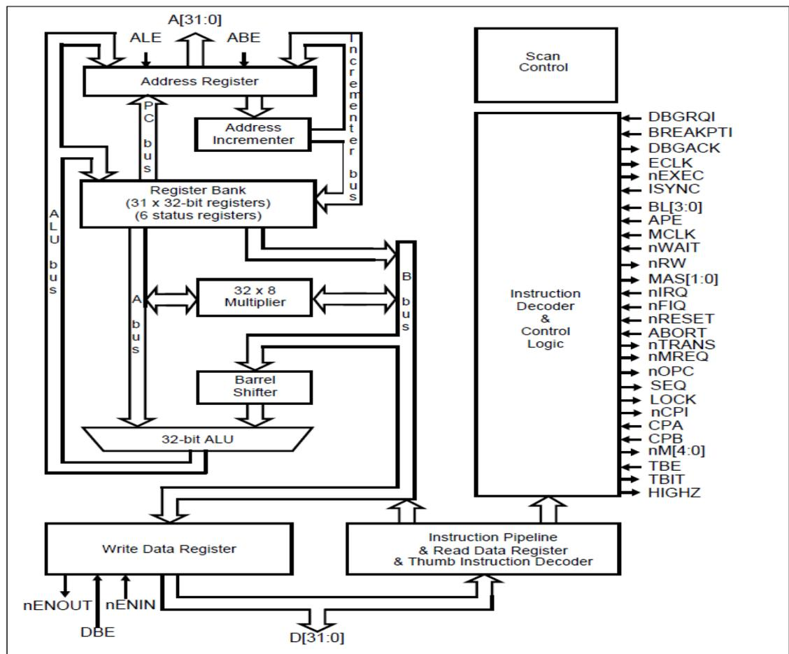
**Figure 4.1:ARM7TDMI Core Diagram**
