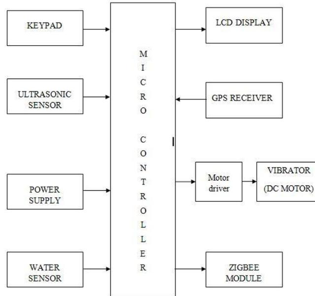
Figure 2.1.1 Block Diagram of Transmitter section in Smart walking stick
