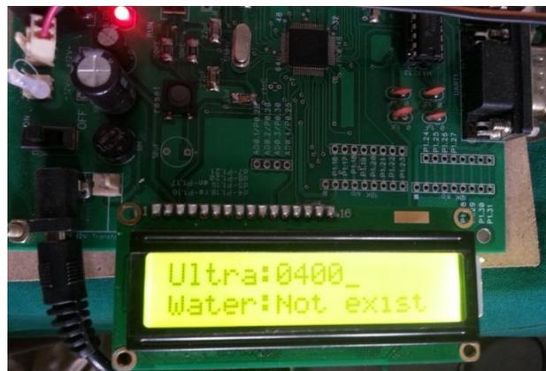
**Figure: Lcd Displayed Values For Sensors measurements**
