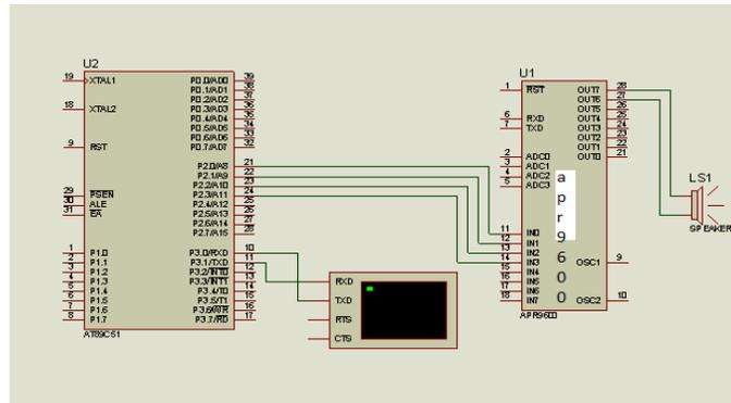
**Figure: schematic diagram for Receiver section in smart walking stick**
