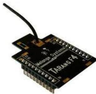
**Figure: ZigBee chip**
