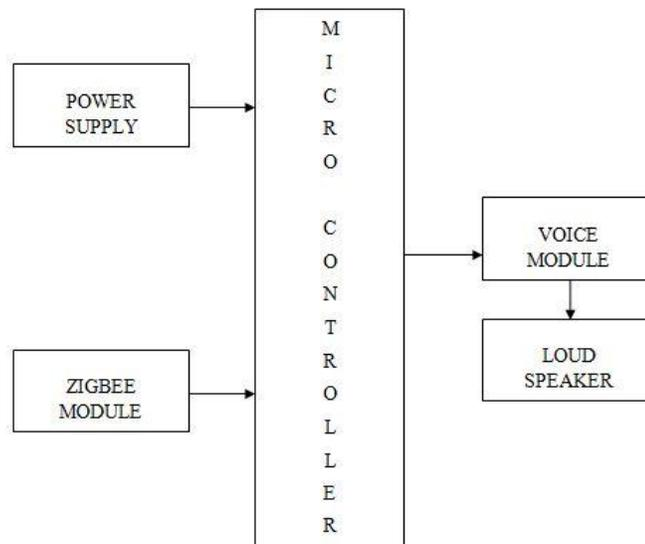
Figure 2.1.2 Block Diagram of Receiver section in Smart walking stick
